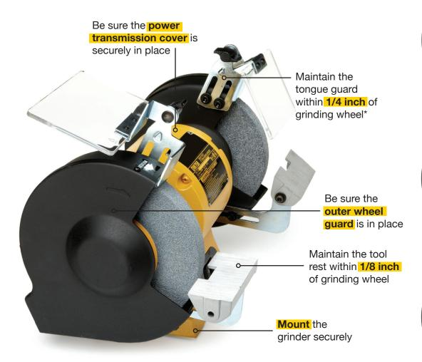
Make sure the manufacturer's recommended speed, as posted on the wheel, is compatible with your grinder
